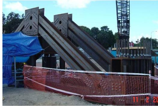
Figure 4: Test pile reaction frame
