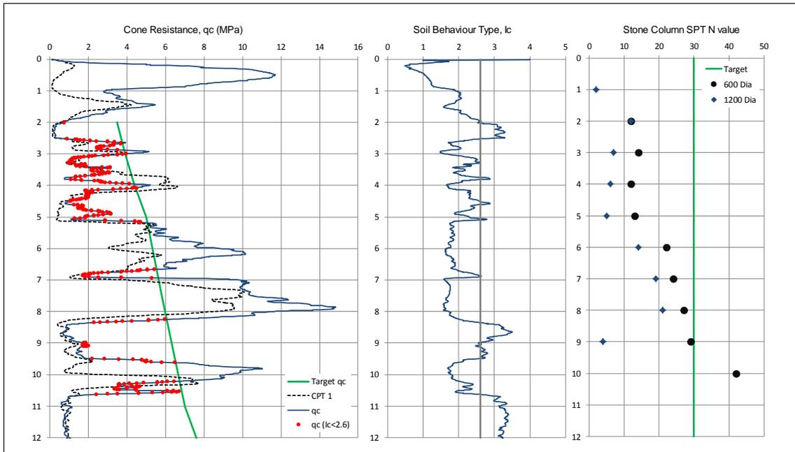
**Figure 3: Test results from columns installed using casing methodology**
