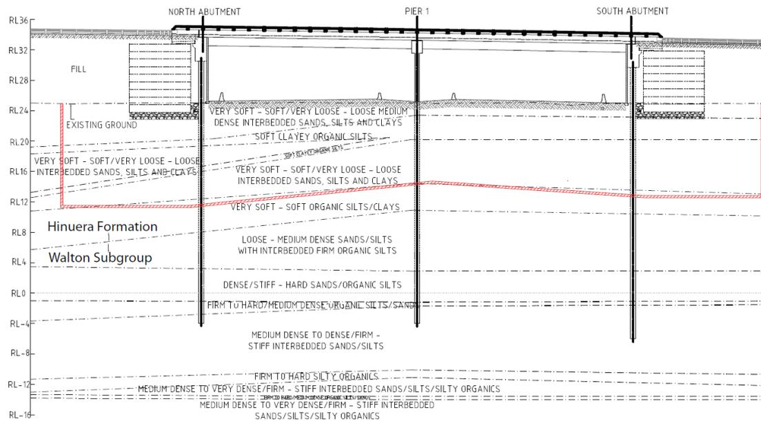
Figure 1: Geologic Profile
