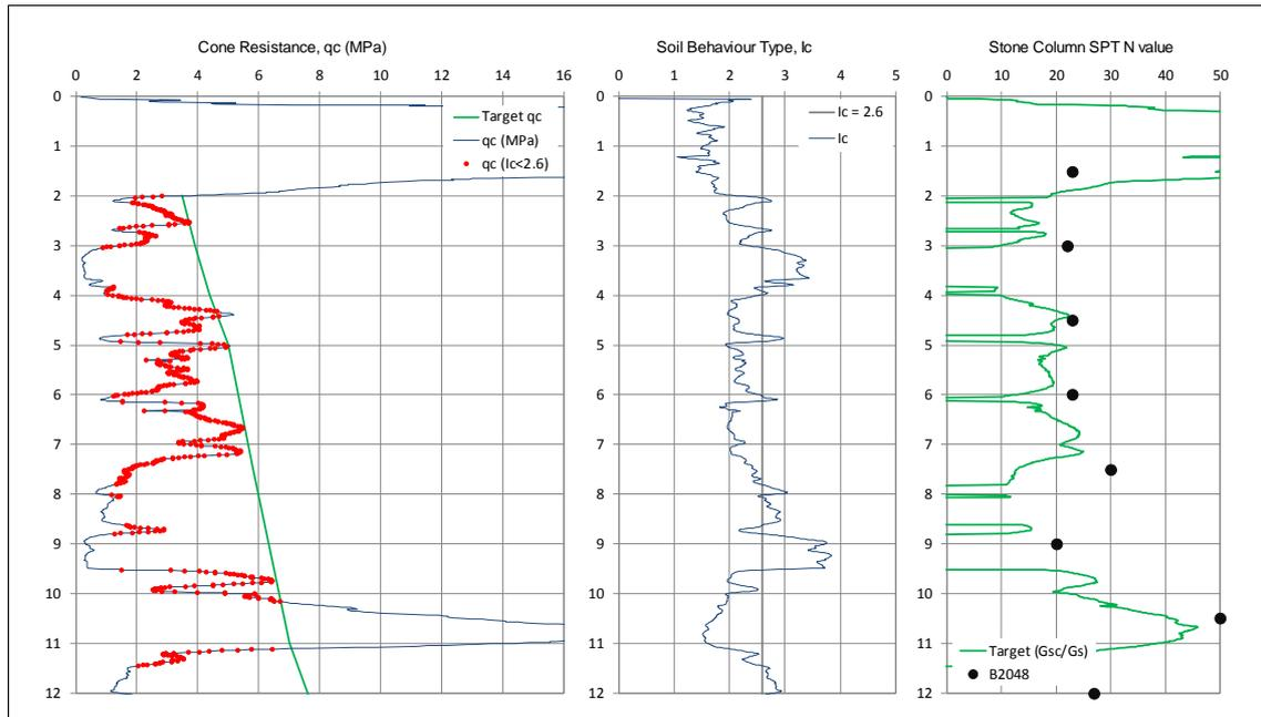
Figure 5: Vibroreplacement Verification
